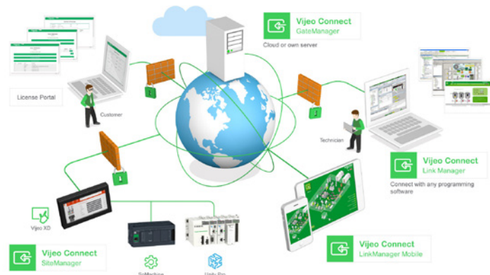
Vijeo Connect for remote programming access to the HMI and its connected devices
